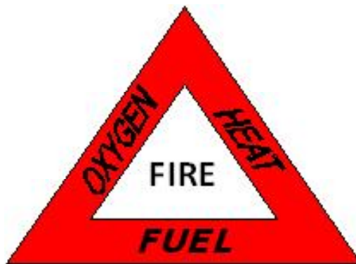
Figure 1.1: The three elements of fire
