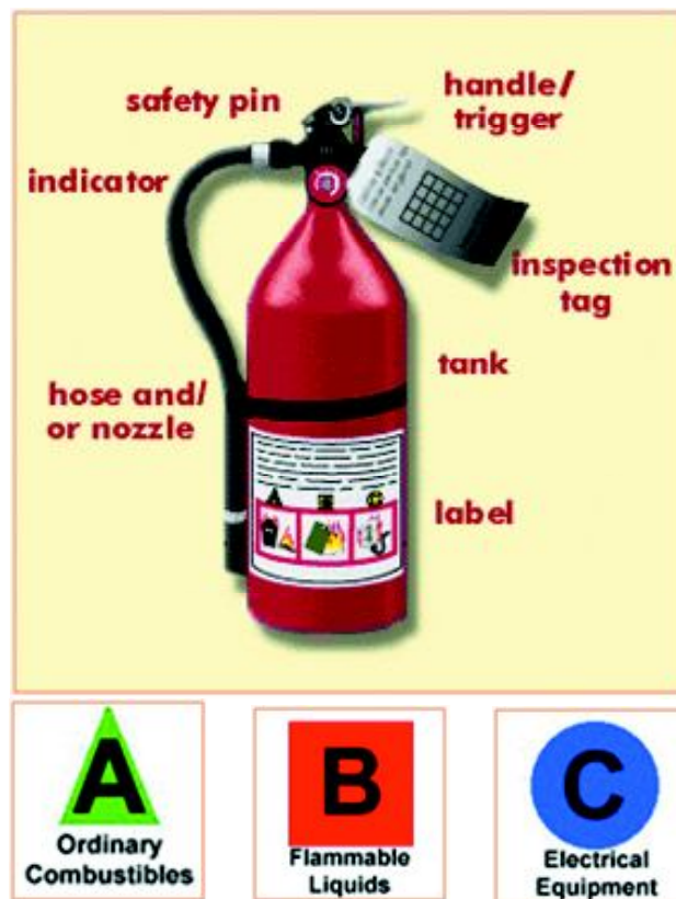
Components of a fire extinguisher
